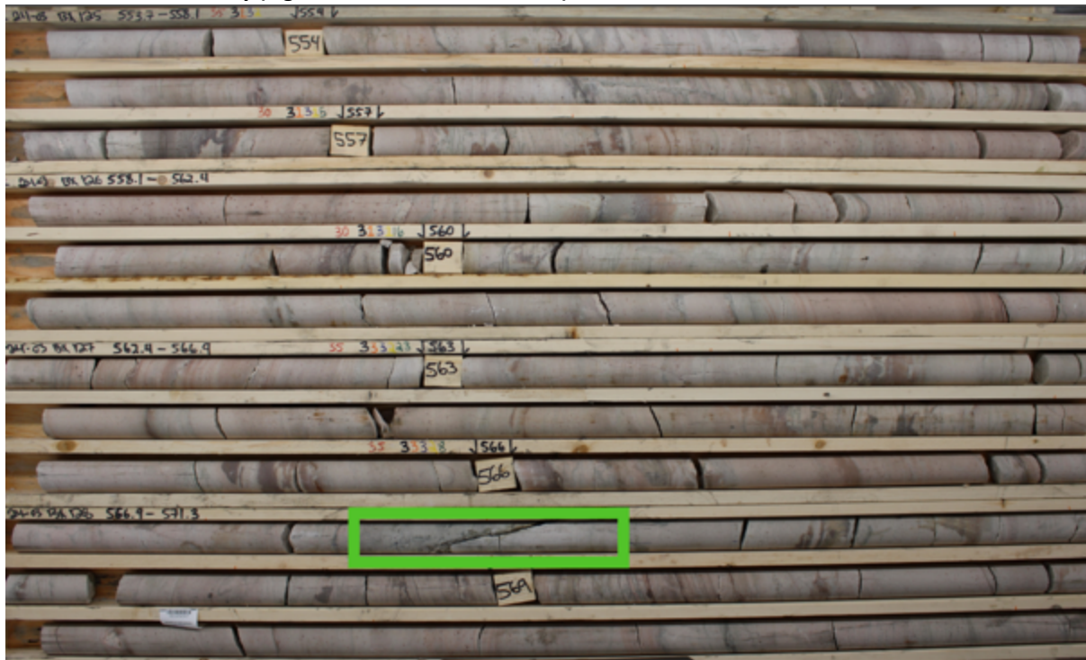
Figure 5 – Pervasively Bleached Sandstone from UR24-03 (553.7 – 571.3 metres) 450 metres above the sub-Athabasca Unconformity (Figure 6 Area Shown in Green)
