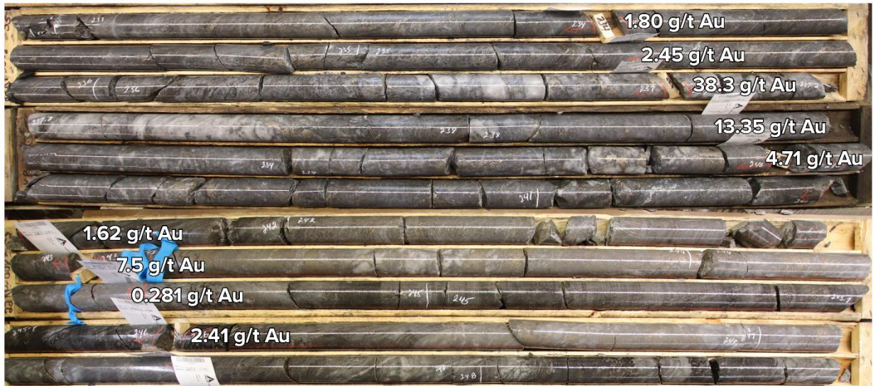
Figure 4: Core photo from 22KP-008 depicting the strong silicification and abundant sulphides typical of the Percival style of mineralization.
