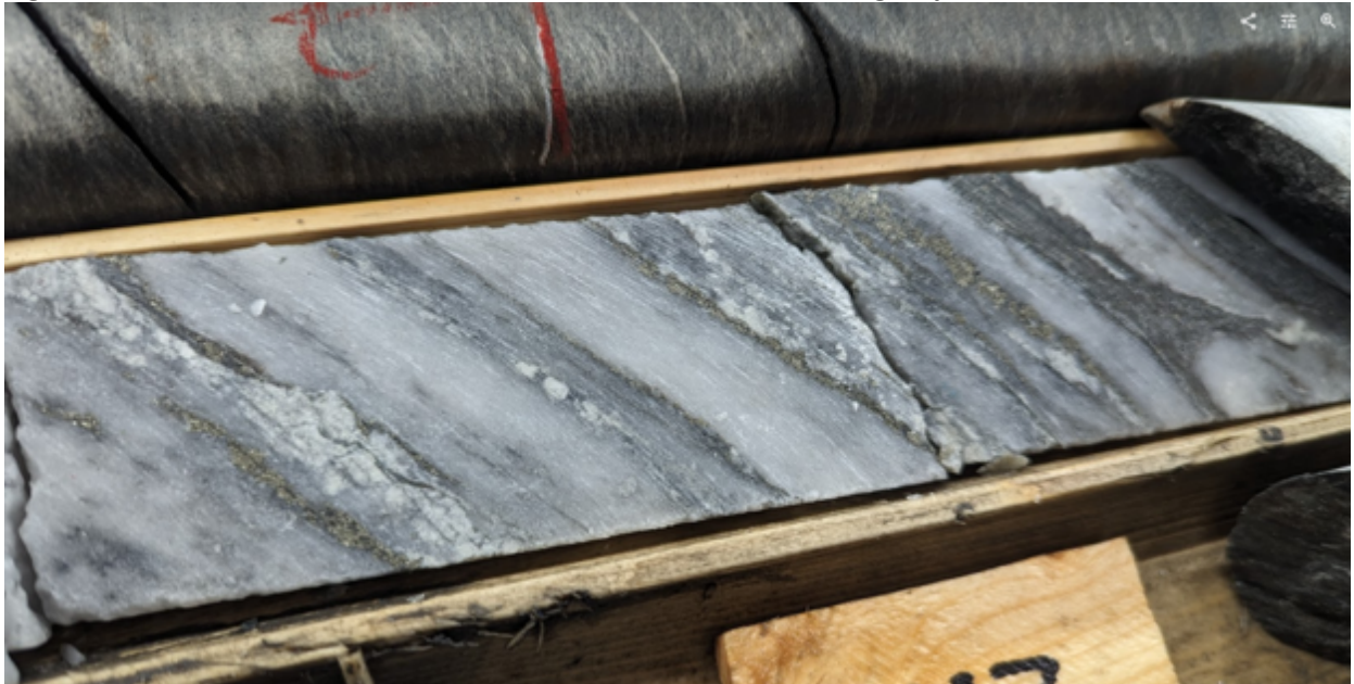
Figure 3 - Photo of laminated vein from Hole GTCM23-055 showing sulphide mineralization:
