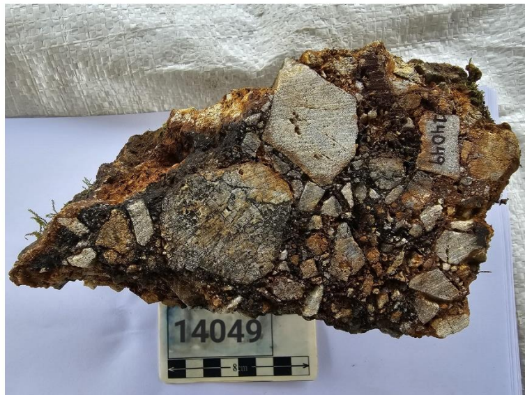
Figure 4b. Sample 14049. Large Boulder 0.5m x 0.45m , hydrothermal gossanous breccia, angular quartz clasts with scattered pyrite and chalcopyrite traces. Matrix filled with oxfe Goe>Jar>Hem, Neotocite filling fractures. Laboratory assays: 1.6 g/t Au, 0.07% Cu, 187 ppm Mo, 0.06% V
