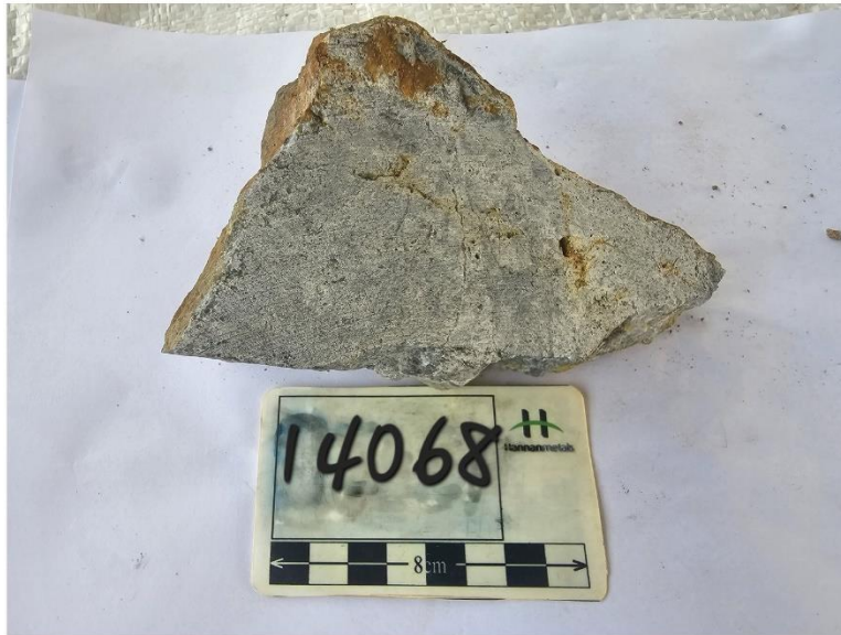
Figure 4a. Sample 14068 porphyritic boulder with phyllic alteration (sericite) and thin quartz veins with pyrite and disseminated jarosite. Green roscoelite disseminated and in veinlets throughout in matrix. Laboratory Assay: 0.42 g/t Au, 0.06% Cu, 0.21 % V
