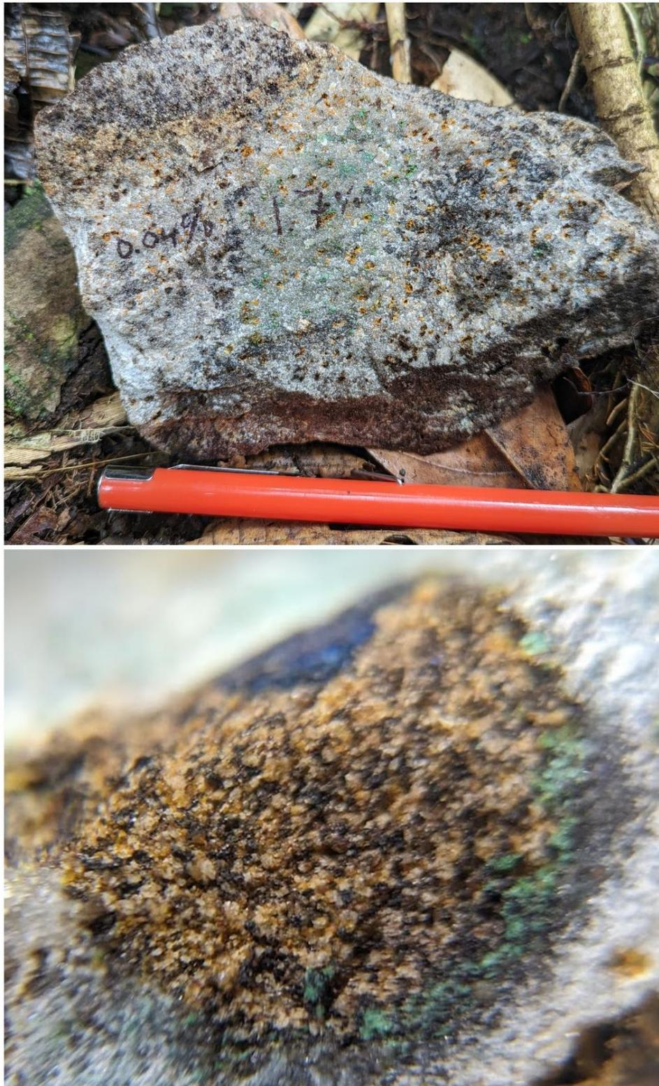
Figure 4. Two photos from channel 869. The top photo illustrates the strong surface leaching of copper sulfide. The white leached surface holds 0.04 % Cu (pxrf) and the partially leached greenish core with copper oxides holds 1.7 % Cu (pxrf).
