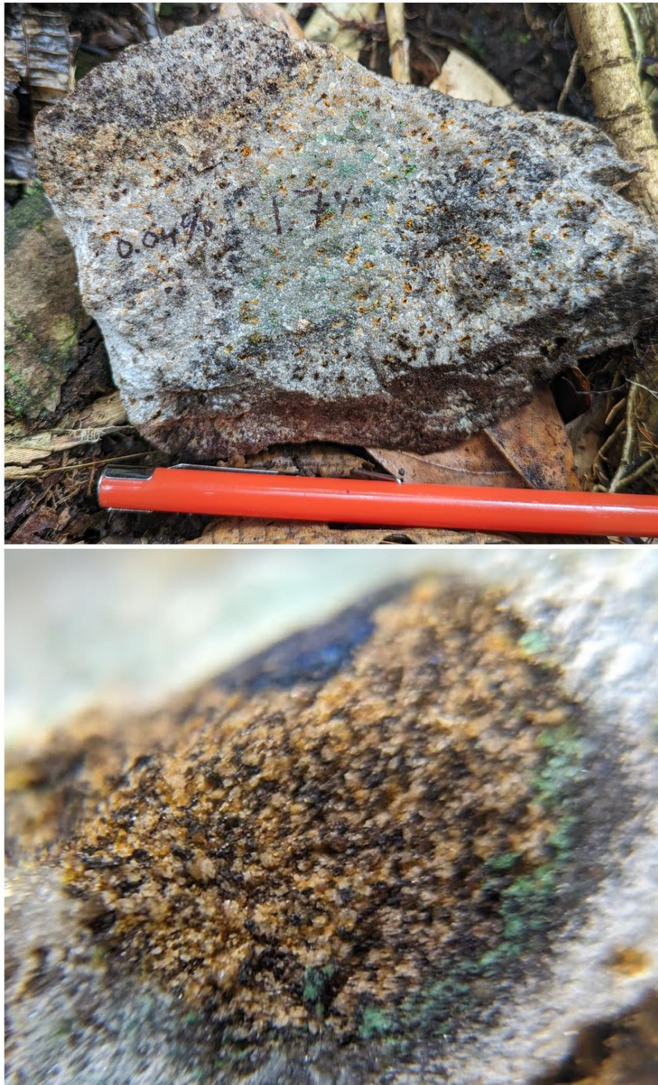
Figure 4. Two photos from channel 869. The top photo illustrates the strong surface leaching of copper sulfide. The white leached surface holds 0.04 % Cu (pxf) and the partially leached greenish core with copper oxides holds 1.7 % Cu (pxf).
