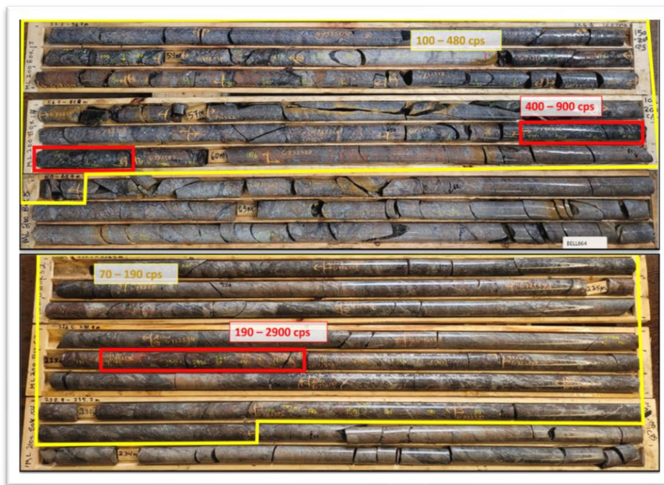
Figure 2: Two zones of typical reddish alteration and uranium mineralization intersected in ML-200.
