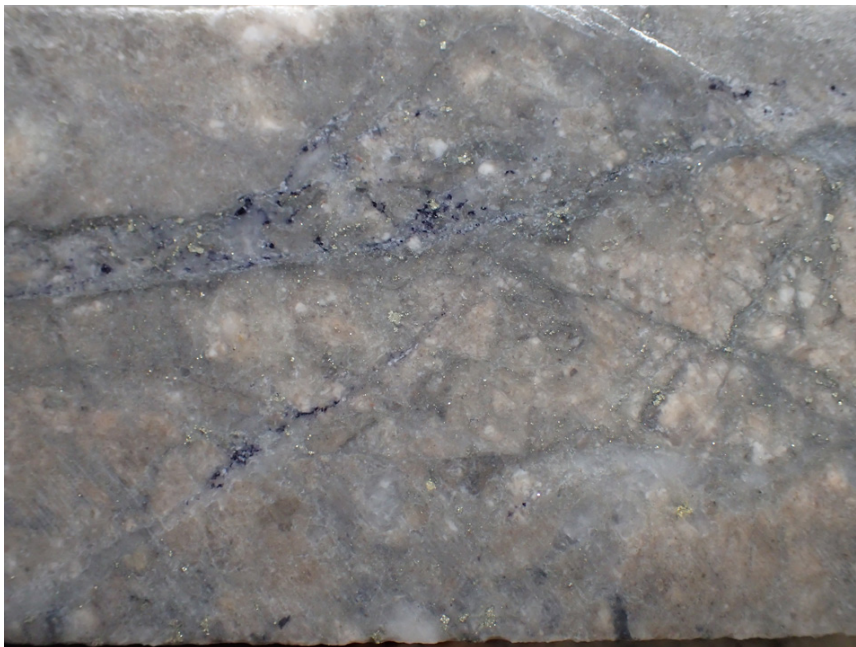
Picture above: Drill-core (DO-18-216) photo from 1.5m interval that returned 86 g/t Au
