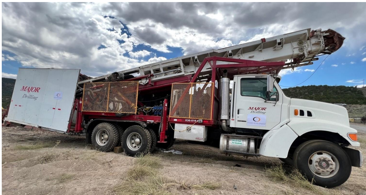
Figure 1: Diamond Drill Rig to Test Copper-Gold-Molybdenum Porphyry Mineralization Potential Arrives at Tintic Project in July 2023
