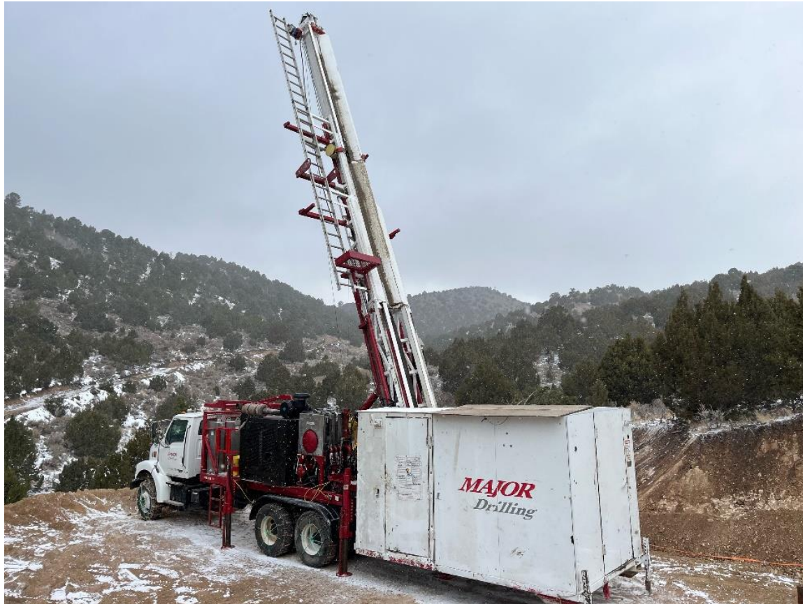
Figure 1: Diamond drill rig to test potential copper-gold porphyry mineralization set up at the Big Hill target at Tintic Project (December 2023)
