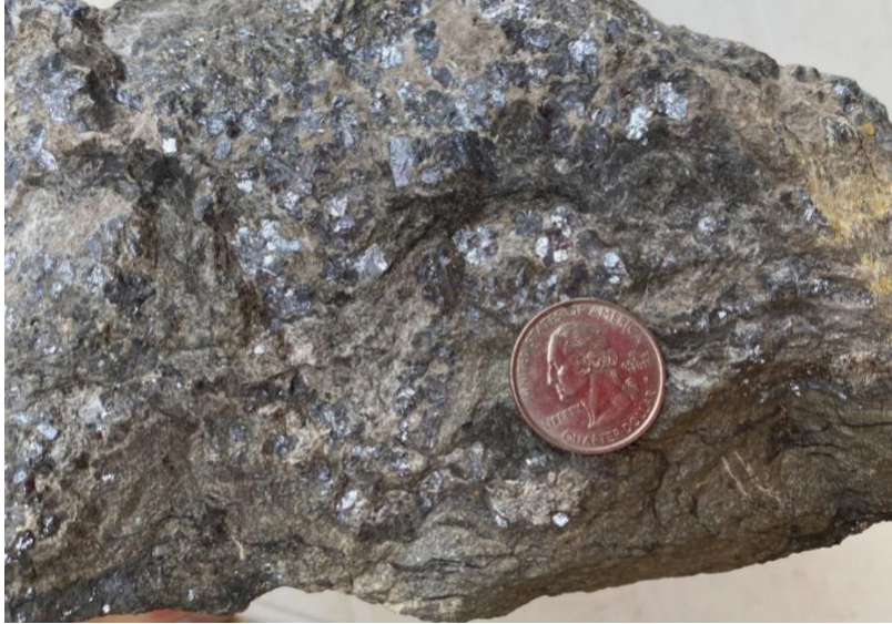
Figure 4. Massive sphalerite (fine-grained, brown) and galena (gray metallic) from the core of one of the high-grade layers of mineralization at Tiria-Shimpia.
