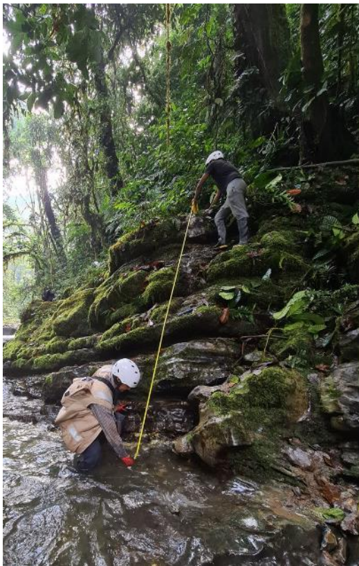
Figure 3. Field teams measuring the true width of mineralized layers exposed in the bank of a stream.
