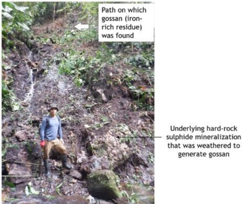
Figure 2. Gossan found on the jungle floor was excavated to reveal fresh, sulphide-bearing mineralization below the weathered layer at Shimpia North.
