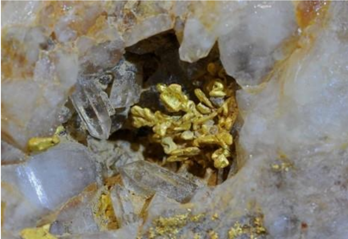
Figure 2: Vug in the quartz vein sample, approximately one centimetre across, containing drusy quartz and crystalline native gold.
