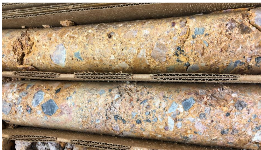
Figure 3. Drill Hole ML20-149CT CIZ diatreme breccia (6.8m @ 4 g/t Au & 1.2 g/t Ag)
