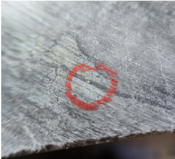
Photo 1 – VG in Con Shear core at 902.7 metres
