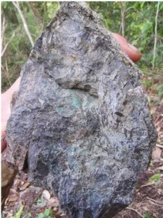
Photo from channel "A" . The sample is characterized by bedding parallel disseminated copper sulphide (chalcocite \text{Cu}_2\text{S} ), in an albitized organic shale host rock.
