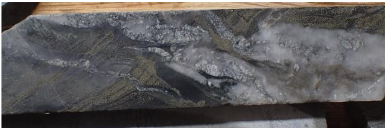
Plate 1: Drill core from EM-22-009 at 991.3m; sedimentary interval within microgabbro unit, in 1m interval that graded 6.66 g/t Au. Note quartz-ankerite veinlets cutting sulfide bands. Visually similar to historically mined mineralization but located well to the north of the main Eagle mine horizon.
