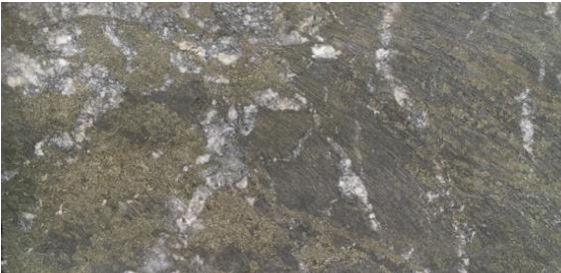
Plate 2: Eagle-Telbel style semi-massive pyrite with fewer iron carbonate veinlets from 352.3 m in EM-22-005, part of a 1 m sample grading 7.6 g/t Au.
