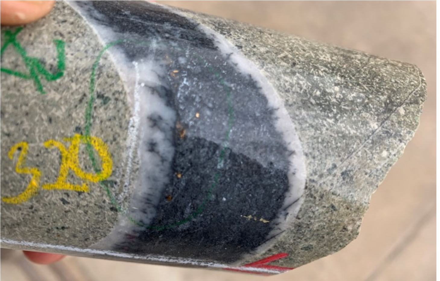
Photo 1: Drillhole MDDSC005 at 130.9 metres showing visible gold grains hosted in a quartz-stibnite vein. The interval from 130.9-131.06 metres (0.16 metres length) assayed 3.7 g/t gold (most of the visible gold was left in the unassayed core). Scale of core is HQ drill core (63.5 mm diameter).
