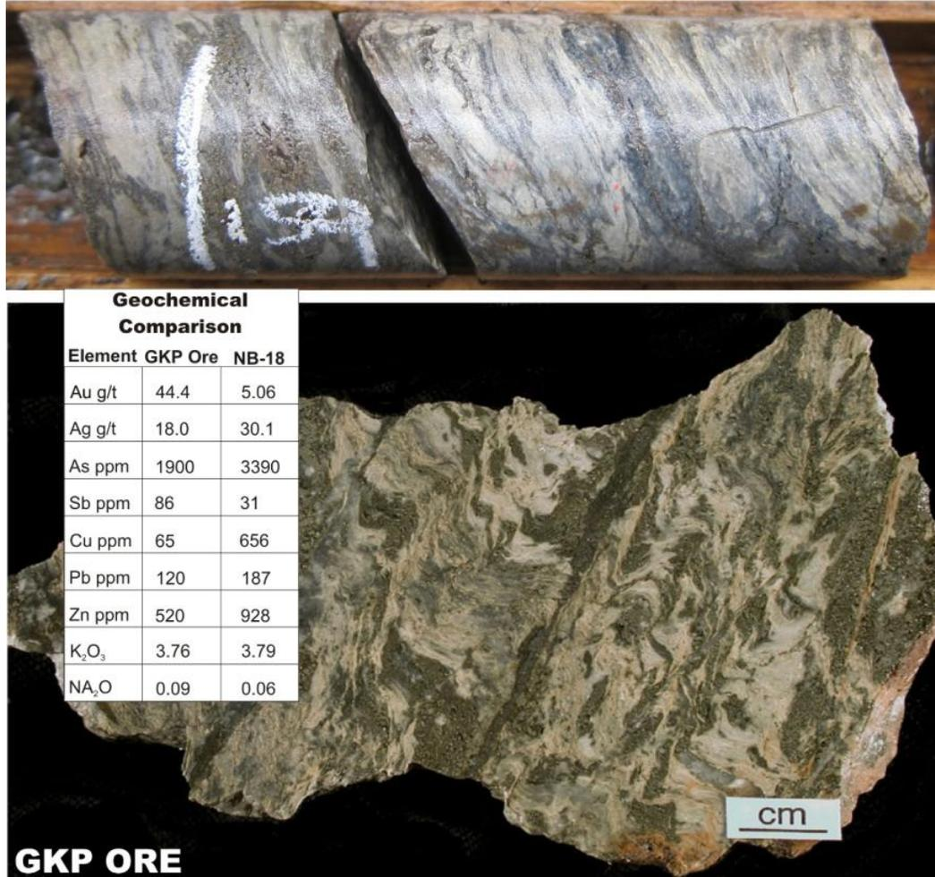
**Figure 2** – Core from the gold mineralized zone in hole NB-18 shows identical shear structure, associated minerals and alteration chemistry to the GKP mine ore sample, demonstrating the extension of this style of mineralization onto TerraX's property. Of note are the distinctive potassic alteration ( $K_2O_3$ ) and sodium depletion ( $Na_2O$ ), with the accessory metals that characterize the Giant Mine ores types.
