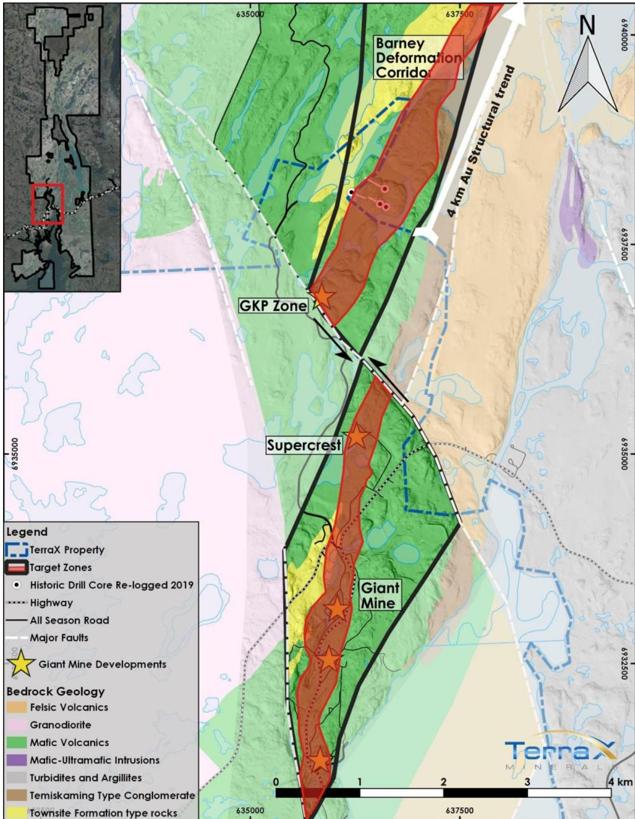
**Figure 1** – Location of relogged and sampled drill holes on the North Giant Extension within the Barney Deformation Corridor (BDC) on TerraX's property. The relogged core area is shown as an extension of the GKP mine, which is the faulted extension of the Supercrest deposit, which was the highest grade gold deposit from the Giant Mine.
