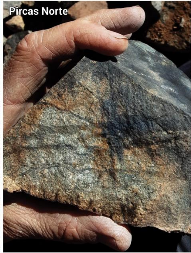
Figure 3: Illustrates depicts typical banded quartz – magnetite – pyrite veinlets hosted within dacite and diorite porphyries from the Gemelos Norte and Pircas Norte target areas, respectively.
