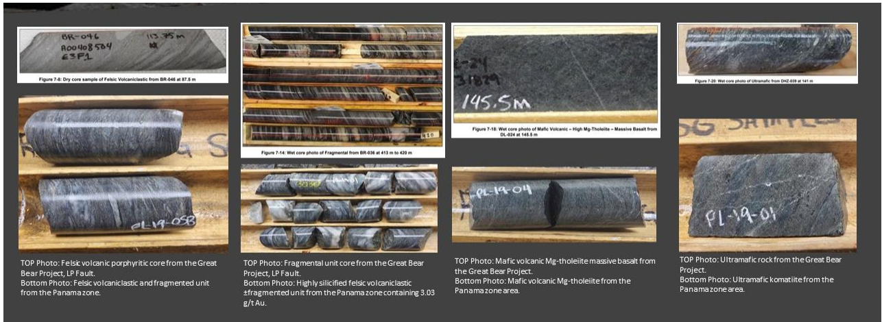
Figure 3: A comparison of Panama Lake core photos illustrating lithological and textural similarities to rocks from the Great Bear project [Kinross Gold]. Great Bear project core photos obtained from Voluntary National Instrument 43-101 Technical Report; prepared for Kinross Gold, Nicos Pfeiffer, John Sim, Yves Breau, Rick Greenwood, and Agung Prawsono.
