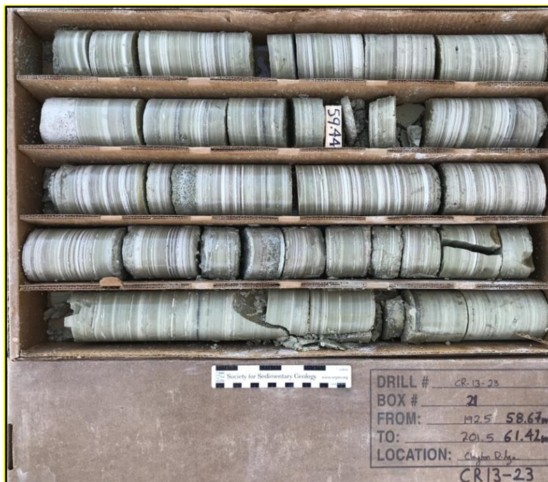
Figure 2. Photo of claystone interval containing 973 ppm Li between 58.7 to 61.42 meters in Hole No. CR13-23.
