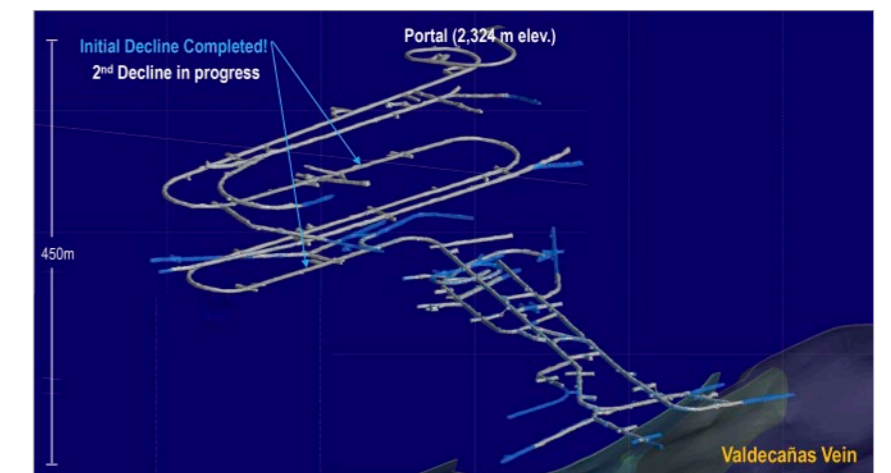
The already built ramp comes up to the upper silver-leading veins. (Source: MAG Silver)
