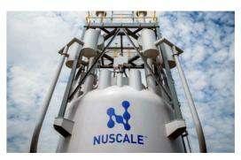
Demonstration model of a NuScale power supply module/small reactor. (Source: Oregon State University/ Wikimedia Commons)
